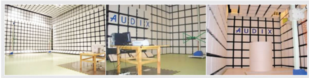
輻射干擾測試實驗室 (10米法半電波暗室) 10m Semi-Anechoic Chamber
